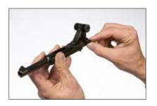
Fold the toggle slightly to relieve tension and remove the retaining pin on the left side. Now pull the toggle joint with breechblock assembly containing the firing pin and extractor back in their guide and out of the frame.
