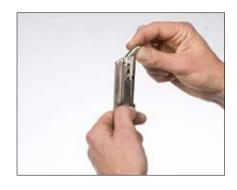
The magazine should only be filled and emptied with the combination tool, which is included with your Parabellum.
