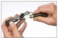
If you wish to remove the firing pin, press firmly on the firing pin spring guide with the combination tool supplied or flat bladed 6mm screwdriver and turn to the left. Then release the pressure to relieve tension on the spring. The firing pin with spring can now be removed.
